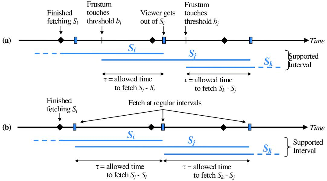
Figure 2: Possible sequences of events in (a) a general spatial and (b) a temporal threshold scheme.
