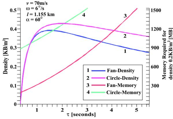
Figure 5: Data density supportable and the amount of core memory required by different pre-fetch duration  $\tau$ .
