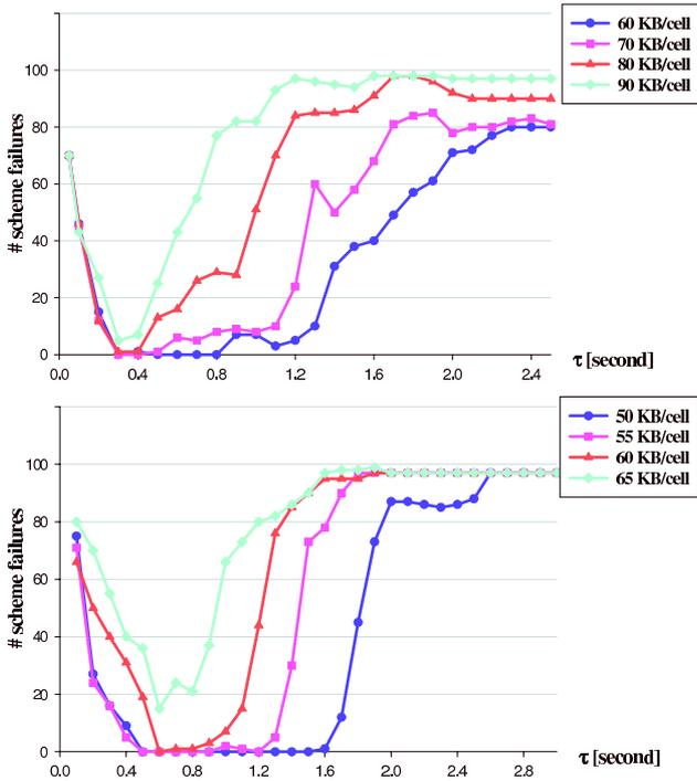
Figure 6: Scheme failures against  $\tau$  with OS disk caching enabled(top)/disabled(bottom) for SCSI-2.8/IDE-2.1
