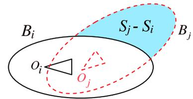
Figure 1: At time  $t_j$ , the pre-fetching scheme decides to fetch  $S_j$ . As some part of  $S_j$  is already in memory, pre-fetching is only needed for  $S_j - S_i$ . Note that the two triangles represent the view frustums at  $O_i$  and  $O_j$ , respectively.
