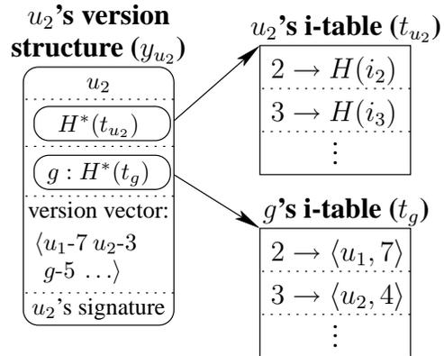
Figure 3: A version structure containing a group i-handle.
