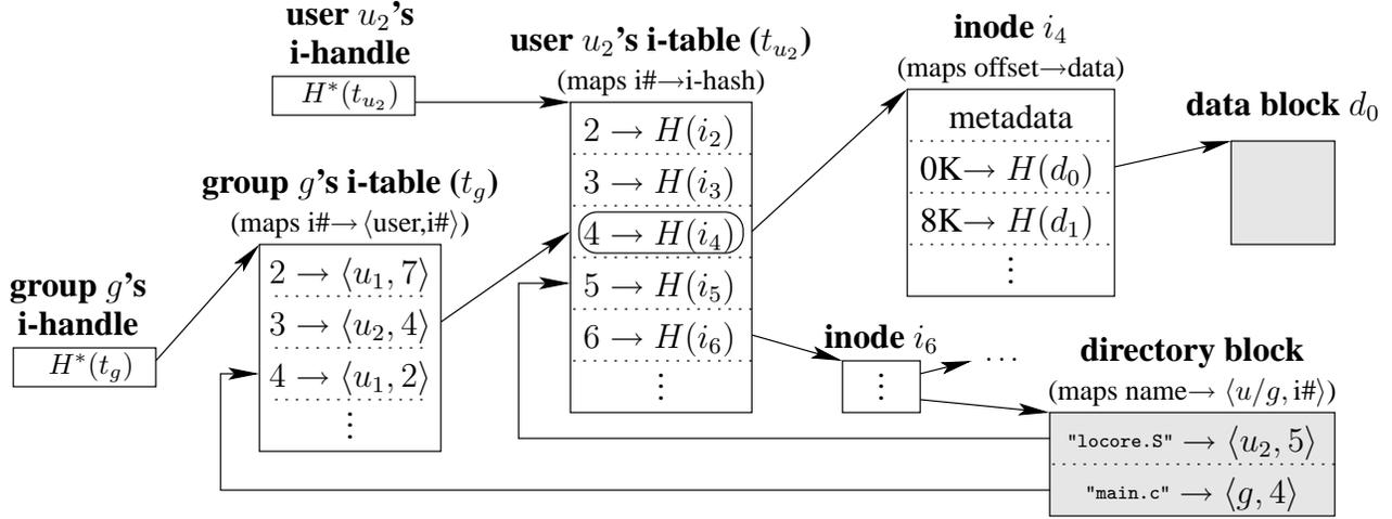
Figure 2: User and group i-handles. An *i-handle* is the root of a hash tree containing a user or group *i-table*. ( $H$  denotes SHA-1, while  $H^*$  denotes recursive application of SHA-1 to compute the root of a hash tree.) A *group i-table* maps group inode numbers to user inode numbers. A *user i-table* maps a user's inode numbers to i-hashes. An *i-hash* is the hash of an inode, which in turn contains hashes of file data blocks.
