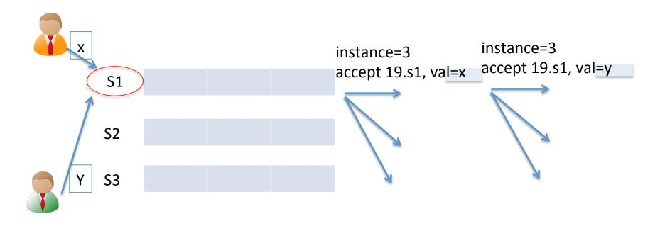
Efficient: leader only needs to run the accept-phase to replicate an operation during normal time
