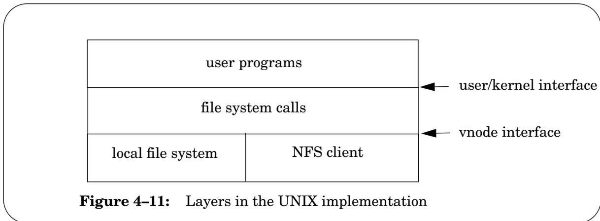
**Figure 4-11:** Layers in the UNIX implementation
