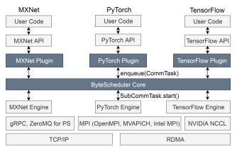
**Figure 5.** ByteScheduler architecture in the communication stack. The dark grey part is added by ByteScheduler.
