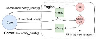
**Figure 6.** Interaction between Core and framework engines without global barrier, *e.g.*, MXNet. Only one DNN layer is shown (assume one tensor in the layer). Operations in squares are added by ByteScheduler. The solid arrows are direct function calls, while the dashed arrows mean dependencies.
